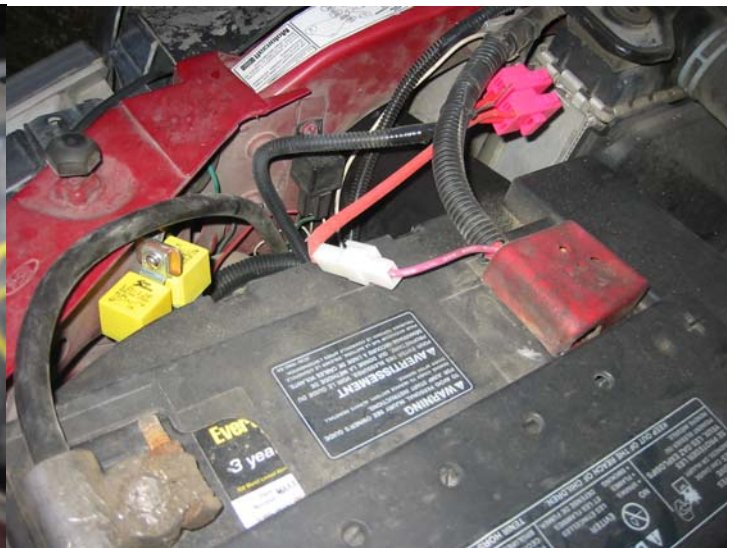
(Water Proof Relays "Yellow" and Battery Connection) (Figure 2)
