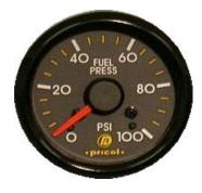
The fuel pressure gauge used on the 7.3L Ford is a 0-100 psi mechanical gauge and needs to be installed using a fuel isolator to ensure diesel fuel cannot enter the trucks interior due to a gauge or tubing failure. Install the gauge into the gauge mount with the tubing connected to the back of the gauge and fittings tightened. Pull the tubing through the firewall and
