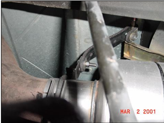
Use standard muffler hanger for rear muffler support details. Stock muffler hanger to be removed and welded to the Walker muffler.
