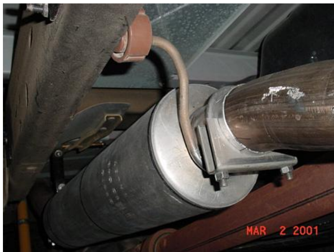
Front mount details, showing the muffer hanger, removed from the stock muffer and welded to the Walker muffer. Also shows the position of the relocated front muffer hanger bracket. The stock front muffer hanger bracket, that was relocated forward, about 12", to support the longer Walker muffer. Use existing bolt hole in the frame.
