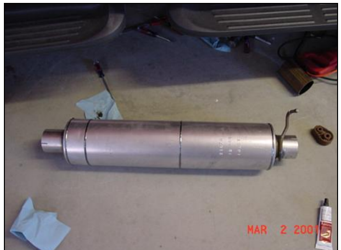
Front muffler hanger welded on (from the stock Ford muffler)
