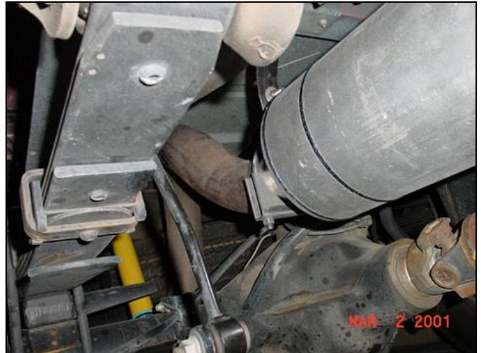
Close up of muffler install, looking back.
