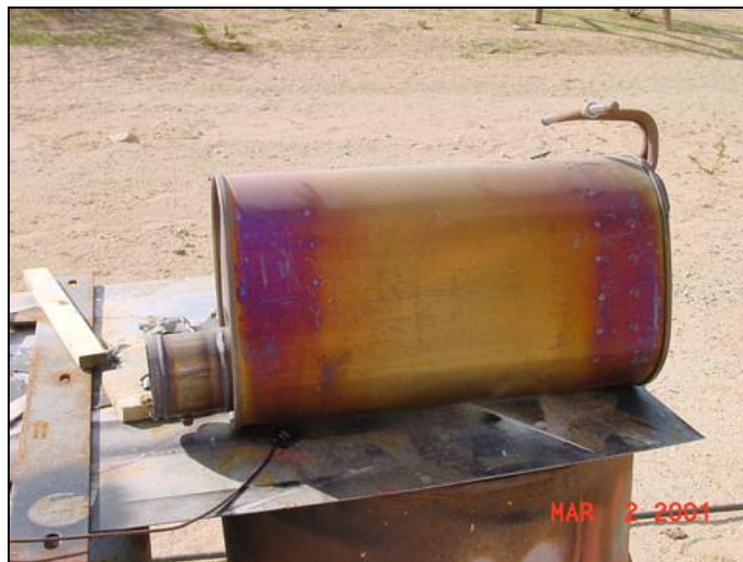
Stock muffler view with inlet on the left. You can see how HOT this muffler got. EGT's have dropped 150F with the Walker muffler.
