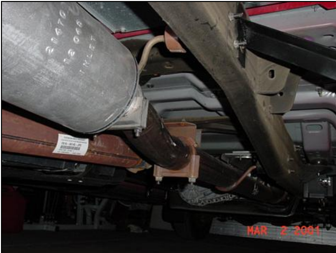
Walker muffler install, looking forward
