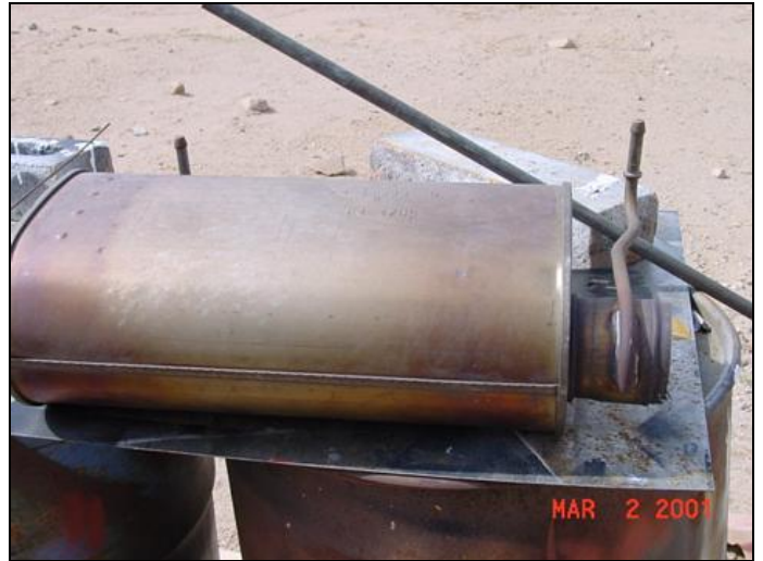
Use standard muffler hanger for rear muffler support details. Stock muffler hanger to be removed and welded to the Walker muffler.
