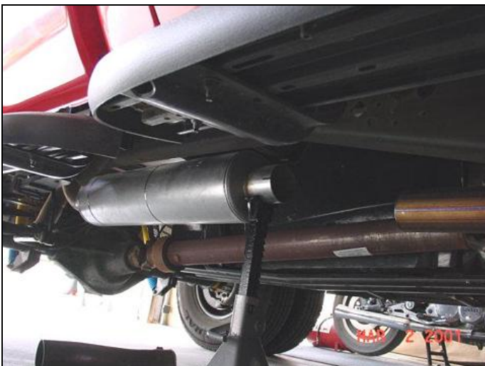
Test Fitting Walker #21470 muffler
