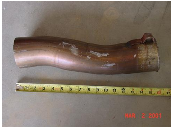
The 'S' bend was rotated 180 degrees The hardest part of the install was getting this piece off the stock system, as the clamp 'crimped' it in place.
