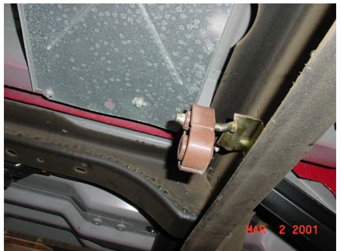
Front mount details, showing the muffer hanger, removed from the stock muffer and welded to the Walker muffer. Also shows the position of the relocated front muffer hanger bracket. The stock front muffer hanger bracket, that was relocated forward, about 12", to support the longer Walker muffer. Use existing bolt hole in the frame.
