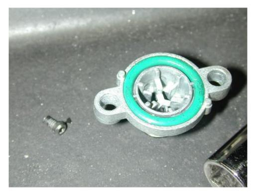
The recess in the center of the cover is where the spring sits. If your putting the spring back in with the shim and do not get it centered into this recess, you'll get about 110 PSI.
