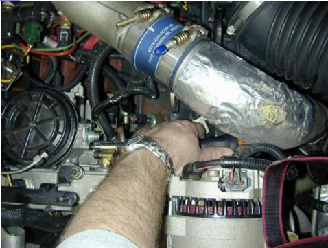
First break the screws loose 1 turn with the T25 Torx screwdriver. I've found it best to use my left hand for this while holding myself up with my right hand on the alternator - unless you are taking pictures with your right hand. Then use you head against the hood for balance.
