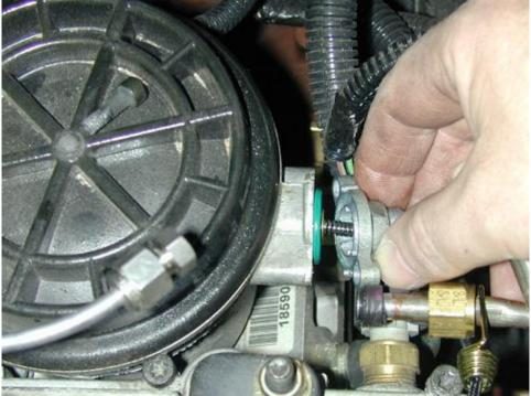
Removing cover: While still keeping the cover tight to the housing with my left thumb, I switch over to my right hand and back the cover off. On this motor the O-Ring stayed with the housing (another part not to drop). There is a lot of spring tension BTW.
