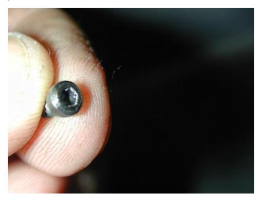
Shim (screw) head: Along with grinding down the head of the screw, I also put a slight chamfer on the edges.
