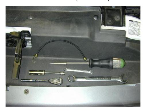
These are all the tools necessary when installing a shim to the OE regulator to increase the fuel pressure. 16mm Open wrench, 13mm socket, 25 Torx bit, and all important bungee cord (metal ends, size unimportant. I also have a 1/4 open end wrench shown, but not necessary. You also need padding because you going to be kneeling on the radiator support killing your knees while praying to the PSD god. - Please don't let me screw this up.
