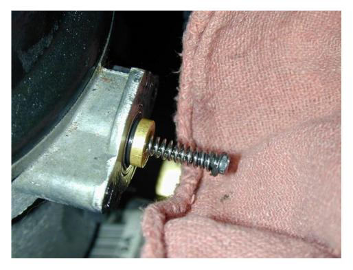
Shim installed: In order to make life easy, I put the screw into the center of the spring with some grease on the threads to keep it in place. Any kind of petroleum grease will work (not silicone), even Vaseline. While I used this shop rag for a photo backdrop, spreading one under this area would be a good idea to catch any of the little parts you may drop.
