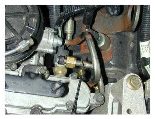
A bungee cord of any size can be used to keep the line away from the cover. The ones with a metal hook end work better then the plastic molded hooks. I've done this way too many times to know that.
