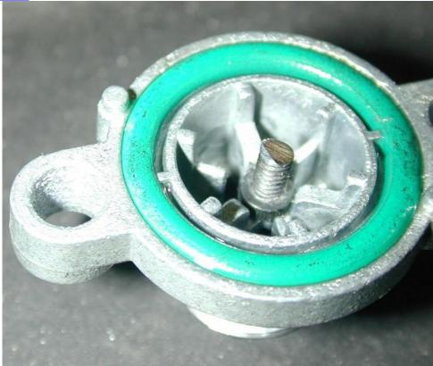
This is how the screw as a shim will fit in the cover. If your using something else besides a 4-40 hex head screw, check it to make sure it bottoms.
