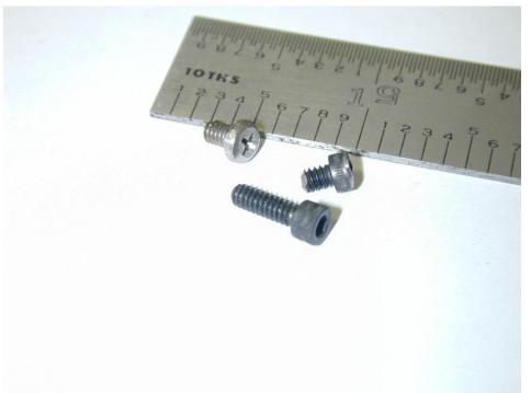
The bottom screw is a 4-40 socket head that is the base material for a shim. At top, I also used a pan head screw, but had to grind down the sides to fit the OE regulator cover. The screw top right has been reworked for 75 PSI. Its head height is 0.075 inch and the threaded section has been ground down to about 3/16 inch so the OE regulator will not bottom out if the filter gets clogged. For reference, a nickel is 0.065 inch thick and 2 dimes 0.090 inch thick if you don't have a caliper
