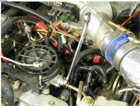
Remove fuel line nut after using the 13mm socket to remove the fuel filter PowerStroke cover, the 16mm wrench is used to loosen the retaining nut from the fuel outlet line. Take note of the position of the original Navistar paint "torque to spec" marking at 12 o'clock.
