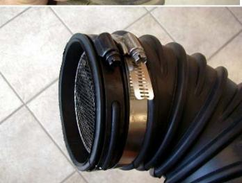
Place the supplied band clamp over the hose as shown in the photo below. Slip the boot back over the turbo inlet using one hand through the boot to guide the TAG into the turbo.
