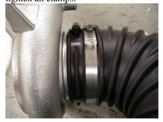
When the TAG is installed properly you should have a gap between the end of the rubber hose and the turbo charger housing as shown in the picture to the left. This gap should be even all the way around.
