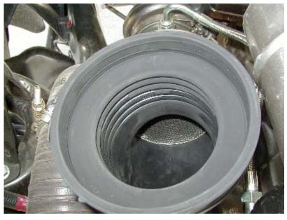
Install the enclosed O-ring on the longer side of the support flange as show in the photo for 2003 - 2005 trucks. The short end will be inserted into the turbo housing.
