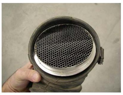
Remove the rubber boot from the turbo charger inlet and insert the TAG into the rubber boot with the longest part of the TAG facing outward as shown. The TAG should snap into the groove inside the boot.
