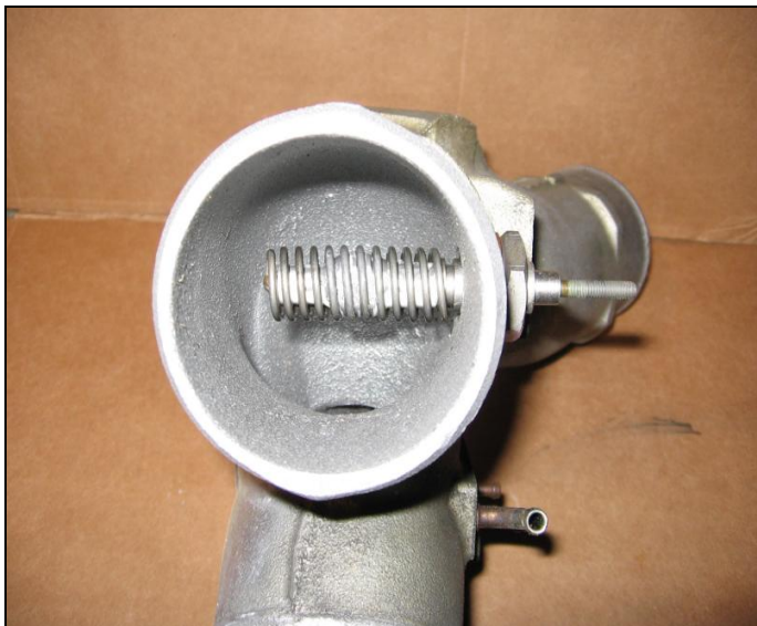
Intake with Heater Installed
