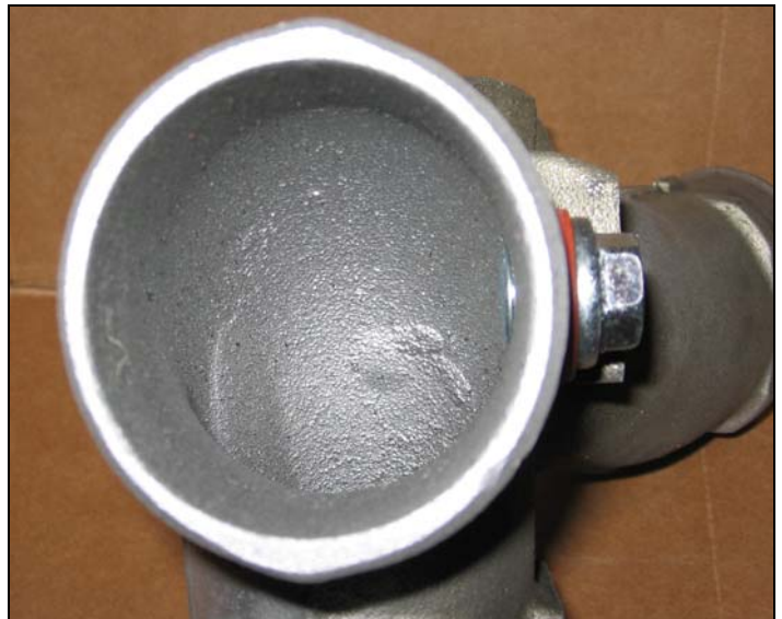
Intake with Heater removed
