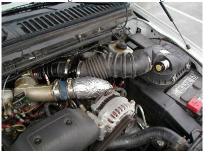
Remove the 4" hose from the air filter housing to the CCV mounted to the valve cover. Then loosen the hose clamps from the tapered hose leading from the CCV connector to the turbo inlet. Remove the two 8mm bolts which hold the CCV connector to the valve cover and remove the tapered hose and CCV connector from the truck.
