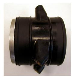
Install the larger TAG into the CCV until the flange stops against the CCV with the shorter end pointing out, towards the tapered hose CCV connection as shown in this picture. Inspect the edges of the smaller TAG for burrs and loose pieces. Even though these parts are cleaned and deburred before shipping you still want to make sure there are no loose pieces which could come loose and be drawn into the turbo. Be sure to wear gloves to protect your hands as some edges may be sharp.
