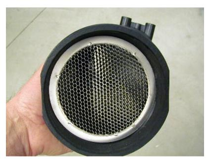
When the TAG is properly inserted into the tube, it should look like the picture to the left. Install the intake tube, air filter hose and all associated connects to complete the job.
