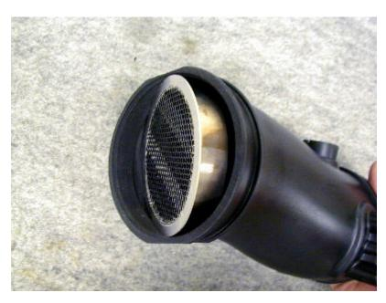
Start the TAG into the tube as shown. Note that the tube has a ridged or recessed area that the TAG will fit into. The TAG is a snug fit into the tube so it may take a couple of tries to get it into the correct position.
